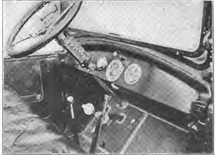
Driver's compartment of the new Overland six, showing left drive and center control, together with mounting of instruments on cowl board
